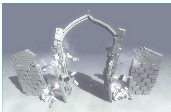
Simulation of a medieval church section failing under seismic loading
